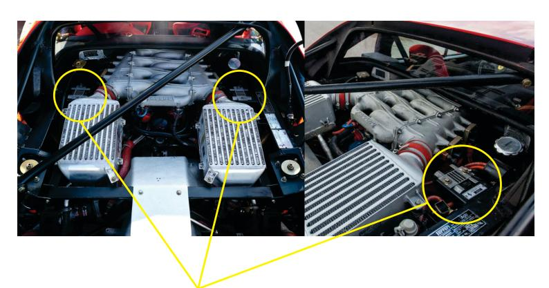
Attach ignition modules in the same location on BOTH sides of the engine bay.
